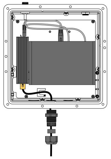
Figure 9: Connecting the network cable
