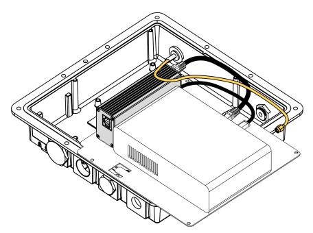
Figure 7: Connecting the antenna connector
