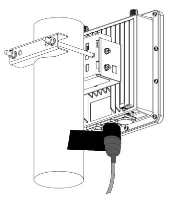
Figure 15: Wrapping with waterproof tape
