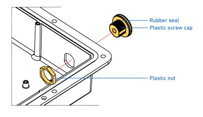
Figure 3: Covering the second antenna hole
