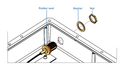
Figure 2: Assembling the antenna connector
