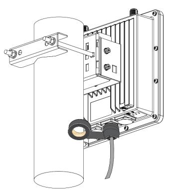
Figure 14: Wrapping with PVC tape
