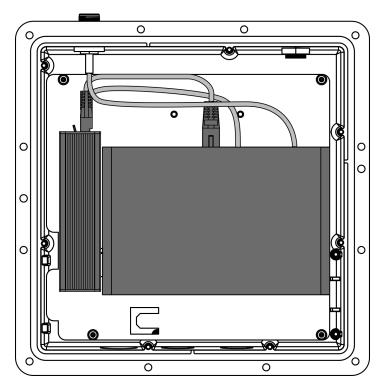
Figure 8: Fixing the miner inside the enclosure
