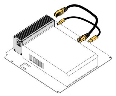
Figure 6: Connecting the PoE Splitter to the miner
