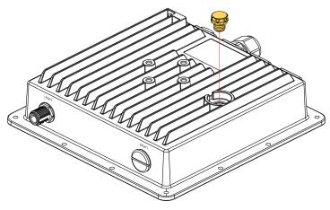
Figure 4: Covering the vent hole
