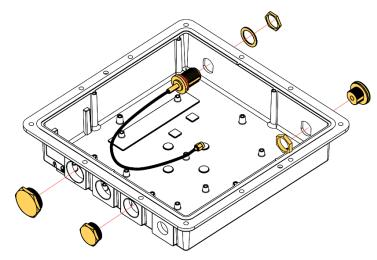
Figure 1: Positioning of all the plugs
