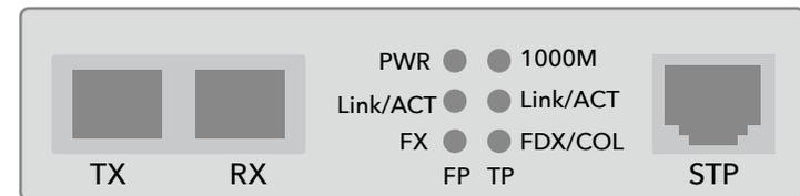
3. Explanation for LED indicator lamp LED indicator lamps serve as device monitoring and trouble display. The following is the explanation for each LED indicator lamp.
