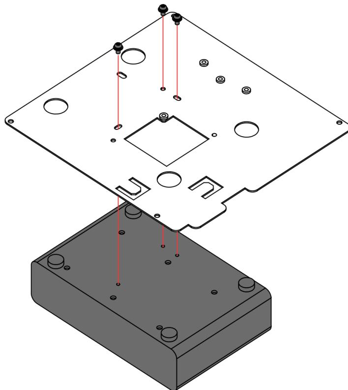
Figure 5: Securing the miner to the plate
