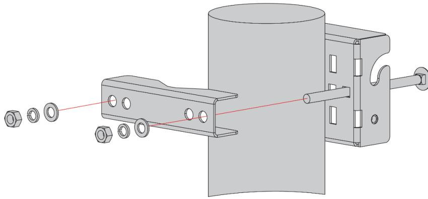
**Figure 11:** Positioning and fastening the pole clamps
