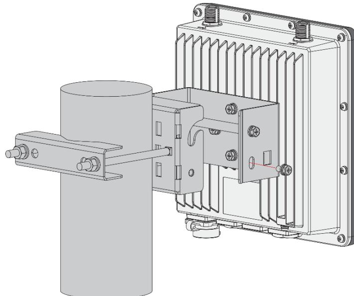
**Figure 12:** Fixing the enclosure to the pole
