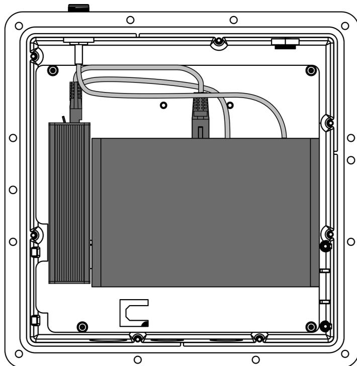
Figure 8: Fixing the miner inside the enclosure
