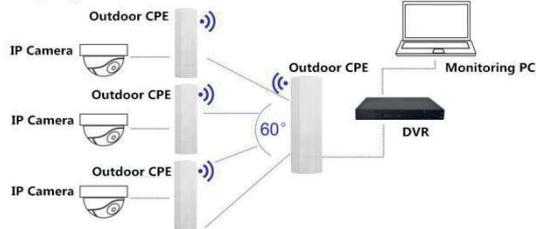
4.PTMP Working Diagram of Outdoor CPE work with Multiple IP Camera
