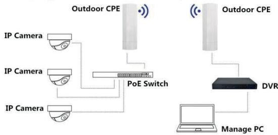
3.PTMP Working Diagram of Outdoor CPE work with IP Camera
