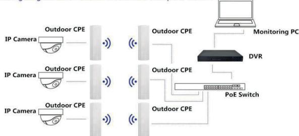
5.PTP Working Diagram of Outdoor CPE applied to Wireless Coverage
